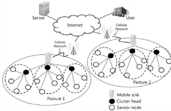
Fig. 1 Architecture of WSN for tracking livestock movements
